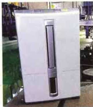
A see-through panel in the door gives a view of the water collected
